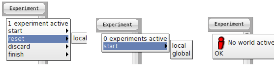
Figure 5.2.: Context menus exposed by the dwdbg debugger extension: During an active experiment, no active experiment and when no world is active (from left to right)
